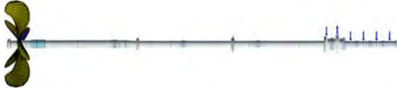
Figure 10: Modelling for shafting alignment
