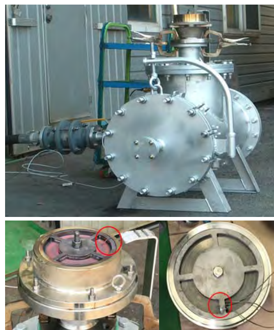
Figure 6: Endurance burning test set-up
