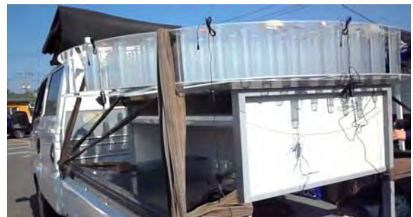
Figure 7: The 2D acoustic Luneburg lens loaded into a small truck. The data outside was taken in this status.
