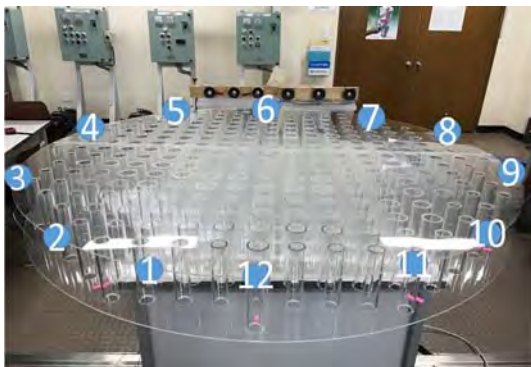
Figure 5: Experimental setup of the 2D acoustic Luneburg lens. The distance between the sound source and the center of the lens is 2,450 mm.
