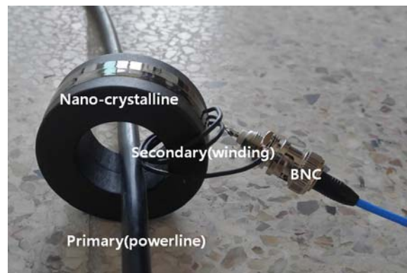
Figure 4: Inductive coupler using a nano-crystalline
