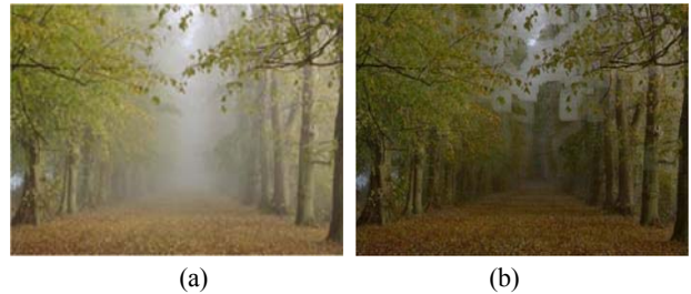
Figure 2: (a) Input fog image (b) Defogging using DCP
