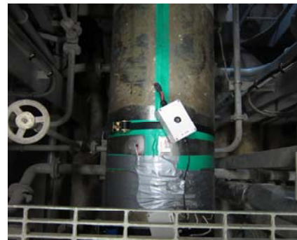
Figure 2: Measurement of shaft force with telemetry system
