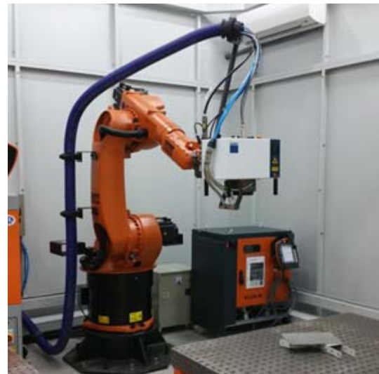
Figure 3: Photographs of 8 kW disk laser experimental equipment with 3D scanner system
