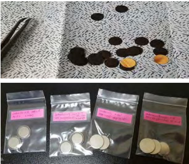
Figure 3: Manufacture of electrode plate and coin cell
