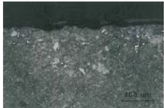
Figure 7: Microstructure of shaft surface section on fretting [5]
