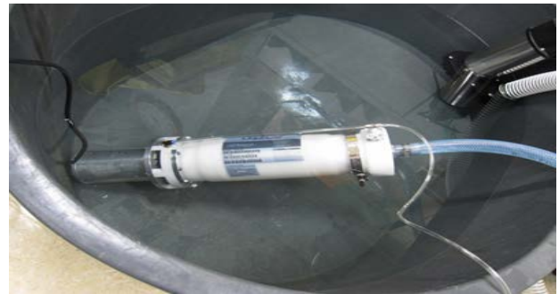
Figure 4: Device for separating dissolved gases from water mixed with exhalation gases
