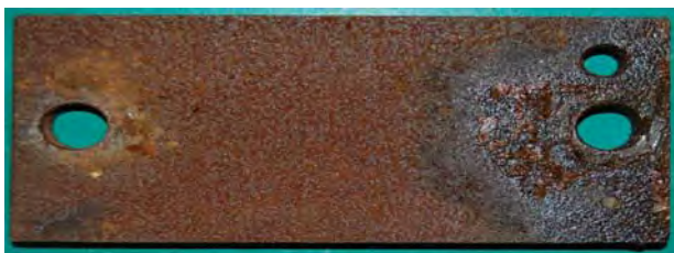
(a) Specimen SS400 before chemical cleaning
