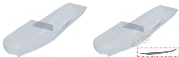
(a) PSV without bilge keel (b) PSV with bilge keel Figure 5: Geometry of PSV
