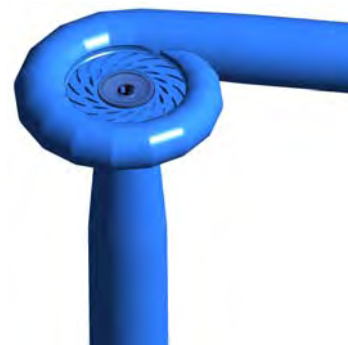
Figure 4: 3D fluid domain of the Francis hydro turbine model for CFD calculation
