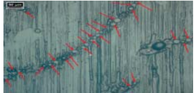
Figure 4: Cat fines embedded into a cylinder liner surface
