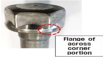
Figure 6: Change in volume of flange in 4th stage to improve flower shape defect
