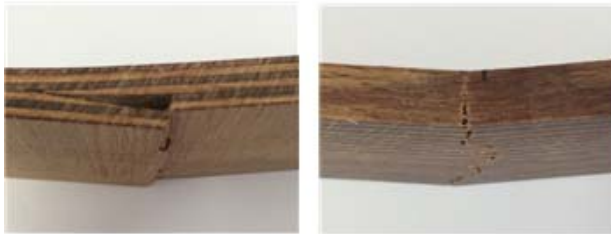
Figure 11: Comparison of the fracture characteristics between CW3 and CW4 at ambient temperature
