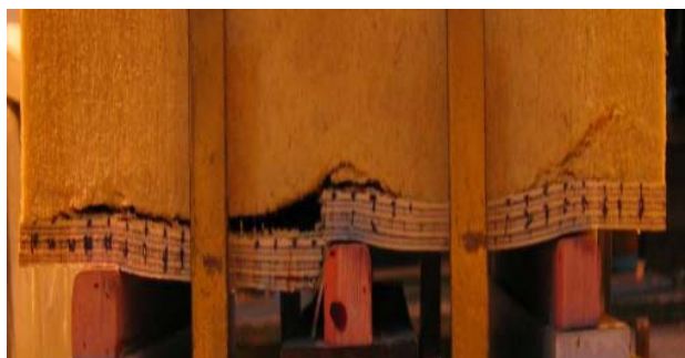
Figure 2: Fracture of plywood in Mark-III
