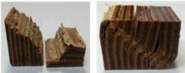
Figure 9: Comparison of the fracture characteristics between CW1 and CW2 at ambient temperature
