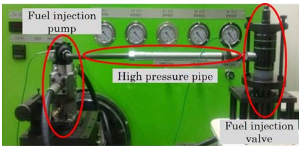
Figure 2: Experimental apparatus of fuel injection system
