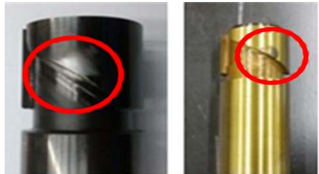
Figure 1: Fuel injection pump components damaged by cavitation
