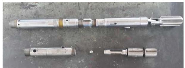
Figure 3: Latch assembly part
