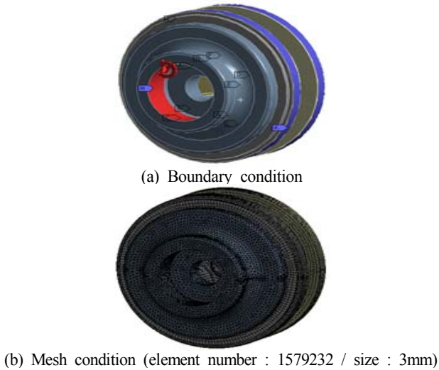
Figure 6: Cycloid cover analysis setting
