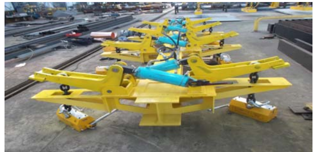
Figure 12: A assembled hydraulic-magnetic clamp
