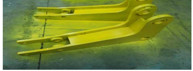
Figure 11: Magnetic arm unit composed of 2 side plates and 1 rib plate to connect the hydraulic cylinders
