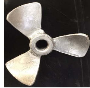
Figure 6: Photograph of axial type 3 blades impeller
