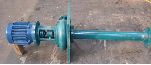
Figure 8: Photograph of the rotor type slurry pump
