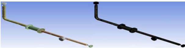
Figure 7: Geometry and finite element model of the whole pipeline model
