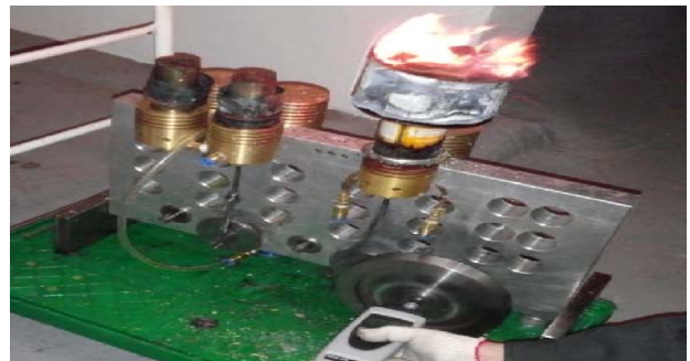
Figure 16: Speed measurements of a typical \gamma -type Stirling engine at 600°C
