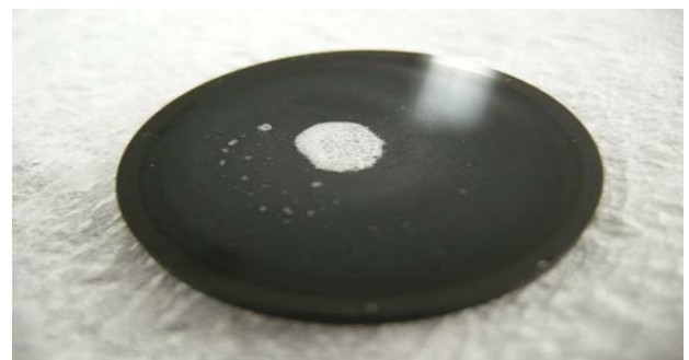
Figure 12: Produced water be white deposits on the optical windows
