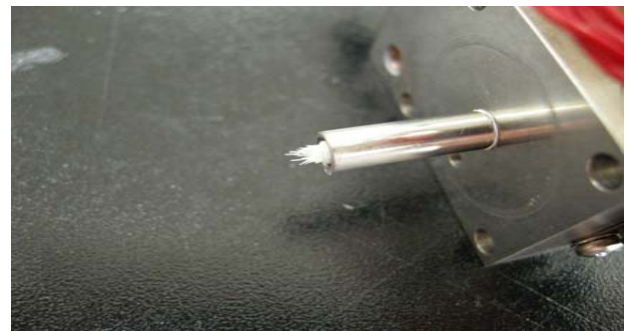
Figure 11: White precipitate was produced in NO x conversion unit
