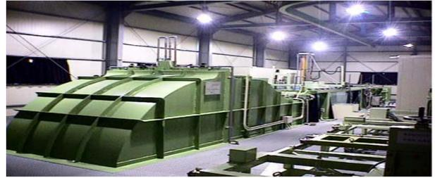
**Figure 9:** A photograph of circulating water channel (Ki (2012) [4] with Permission)
