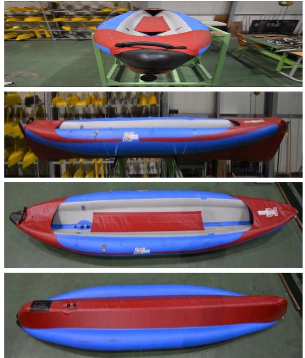
Figure 5: V-hull Kayak (Type 3)
