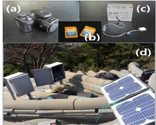
Figure 2: Video monitoring system. (a) Canon Powershot sx500is camera, (b) Eye-fi memory card, (c) 12 V 18 Ah battery, (d) View of camera system setup at the top of the mountain.
