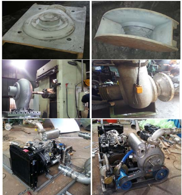
Figure 19: Prototype production of drainage pump system
