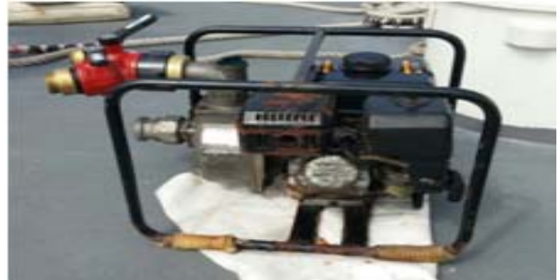
Figure 2: Existing drainage pump of Korea Coast Guard
