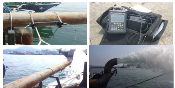
Figure 20: Rate of discharge performance test using the ultrasonic flow meter
