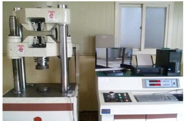
Figure 8: Tension/bending tester-50 ton
