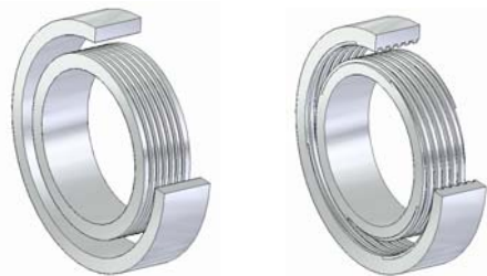
(A) Smooth-Stator/ Parallel-Grooved-Rotor (B) Spiral-Grooved-Stator/ Spiral-Grooved-Rotor
