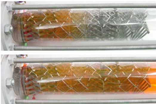
Figure 2: Mixing images with time(of 1 and 2sec) at Re=32,650
