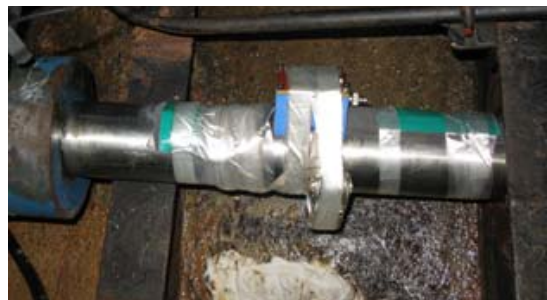
Figure 7: Telemeter system arrangement on 99-mm diameter shaft
