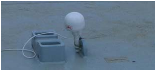
Figure 8: Portable DGPS mounted during speed measurement
