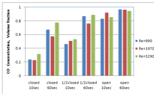
Figure 7: Averaged variations of carbon monoxide concentration predicted in three different tunnel models depending on three Reynolds numbers.
