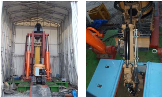
Figure 6: Feature of spiking test system
