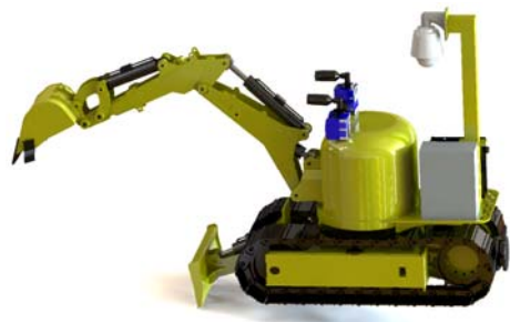
Figure 4: Feature of developed robot controlled by joystick
