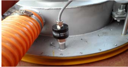
Figure 8: Pressure sensor on the adhesive pad
