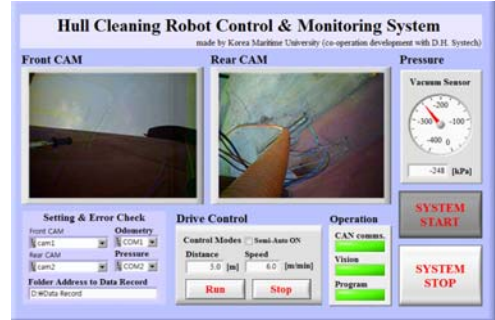
Figure 14: Screen of the control & monitoring unit for a convenient robot operation
