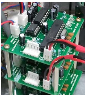
Figure 6: CAN/RS-232 communication converter
