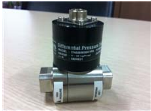
Figure 3: Used differential pressure sensor
