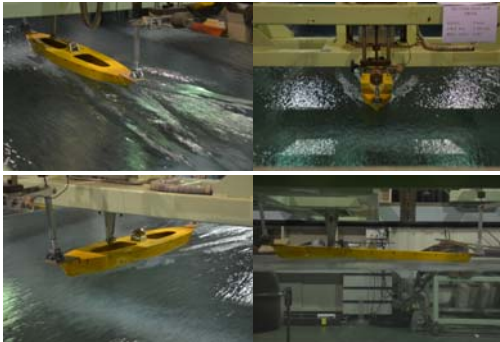
Figure 6: Photographs of Resistance Test (RD-FK-11) : 6.0 knots
