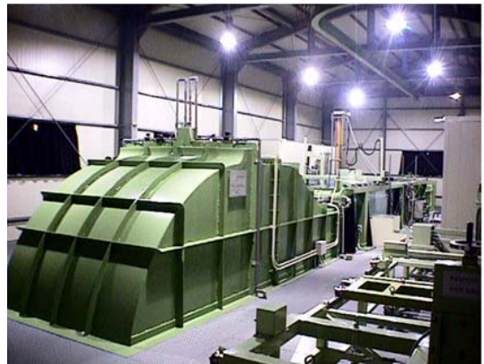
Figure 4: Photograph of Circulating Water Channel (From Ki, 2012, with permission)
