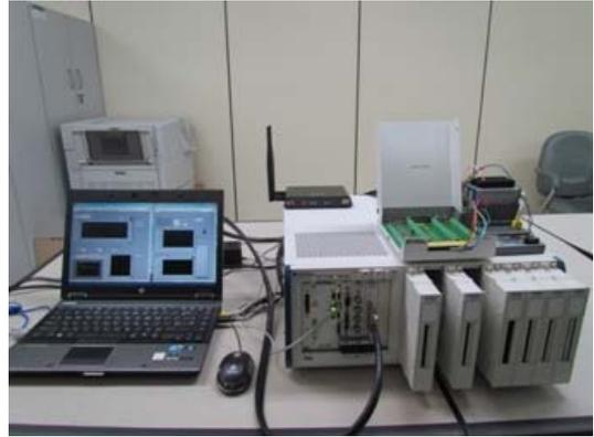
**Figure 3:** Hardware components of HIL Simulator
