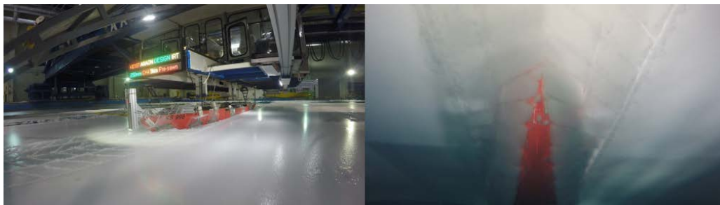
Figure 4: Ice model test in pre-sawn ice (left: above water; right: underwater)
