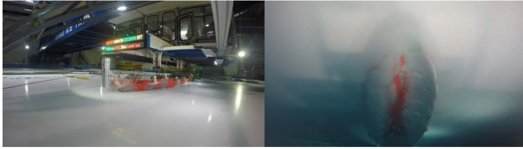
Figure 3: Ice model test in level ice (left: above water; right: underwater)
