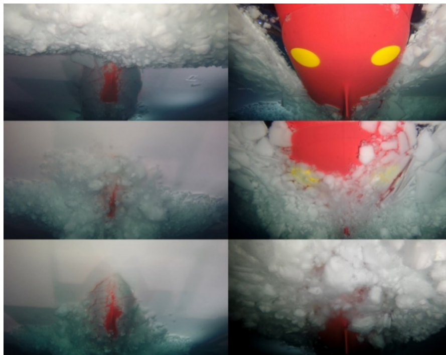
Figure 8: Fish eye's view (top: entering ice ridge; middle: penetrating ice ridge; bottom: after passing through ice ridge)
