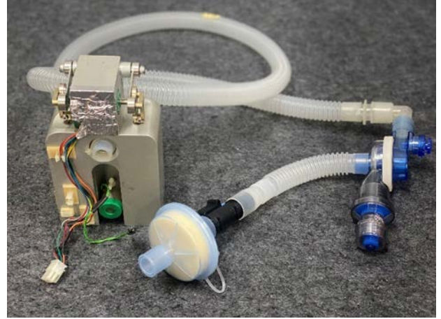
Figure 2: The two double-acting pistons pump in experimental tests.
