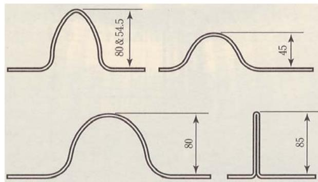
Figure 7 : Corrugation of MARKIII membrane tank
