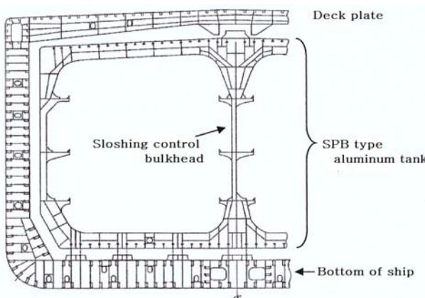
Figure 6 : Central section of SPB LNG carrier
