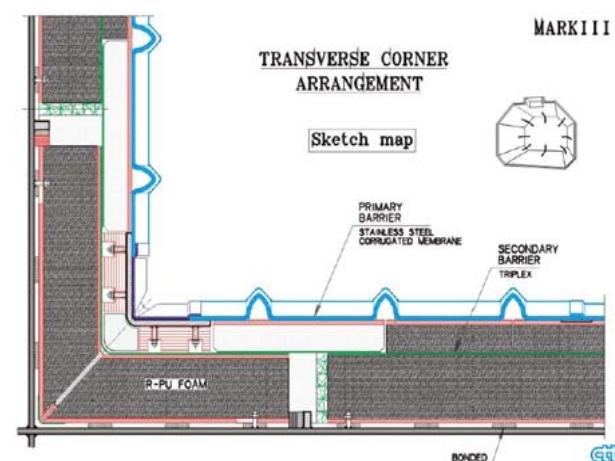
Figure 3: Inner section of MARKIII membrane tank
