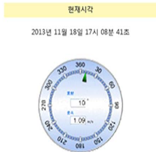
Figure 10: Ultrasonic Wind Anemometer Indicator Layout
