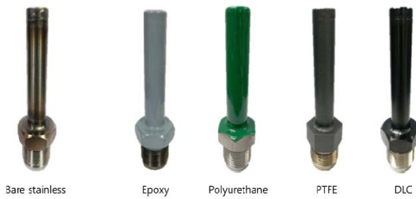
Figure 6: Various cold fingers through processed coating.
