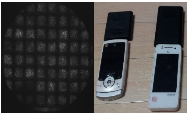
Figure 2: Image of the target grid and two mobile phones. The target is attached onto the mobile phone (model A, model B) for imaging.
