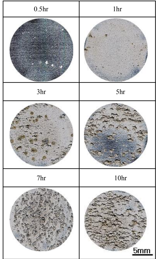
Figure 4: Surface appearances of STS 431 after cavitation test in seawater
