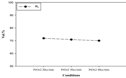
Figure 7: H<sub>2</sub> concentration depending on air supply change of PrOx2 (PrOx1 20cc/min)
