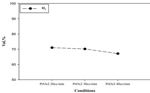
Figure 8: H<sub>2</sub> concentration depending on air supply change of PrOx2 (PrOx1 30cc/min)
