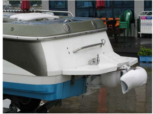
Figure 14: Setup water jet on the boat
